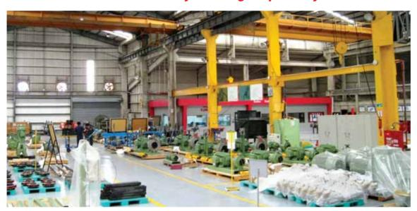
A key component of the facility is the region's largest, most capable hydraulics test bed. Certified testing to API and international standards is provided for both horizontal and vertical pumps (including high-pressure applications) up to 6000 kW (8000 hp). The test bed will allow end users to verify equipment performance or diagnose and correct problems.
